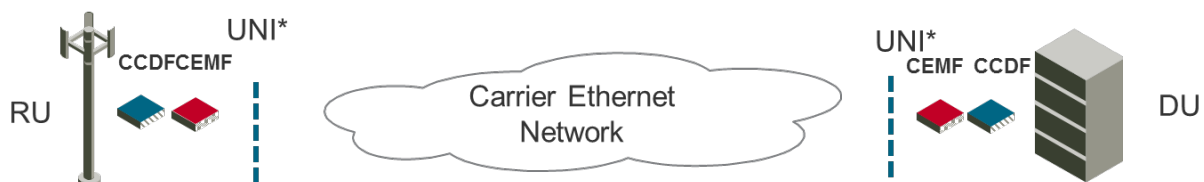
Figure 5-4: Ethernet Service with Compression
