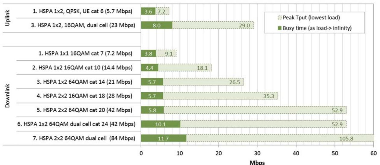
Figure 12: Backhaul Traffic Characteristics HSPA Small Cells in various configurations
