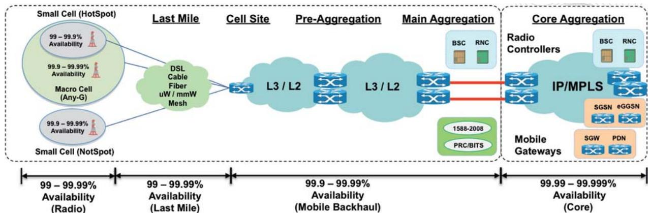
**Figure 15 Availability on each section of the end to end connection**
