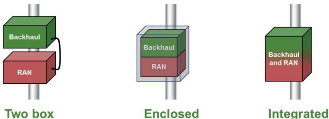
**Figure 16: Levels of integration between a small cell and a transport equipment deployed in the same outdoor location**
