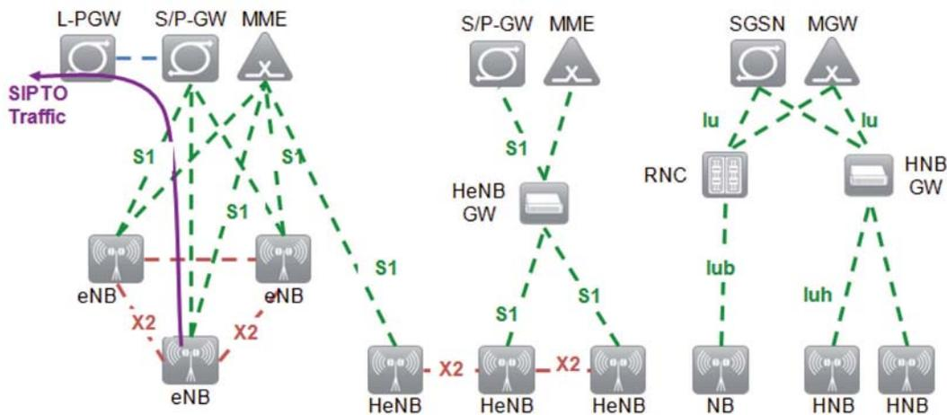
**Figure 2: 3GPP LTE and UMTS Release 10 Architecture**
