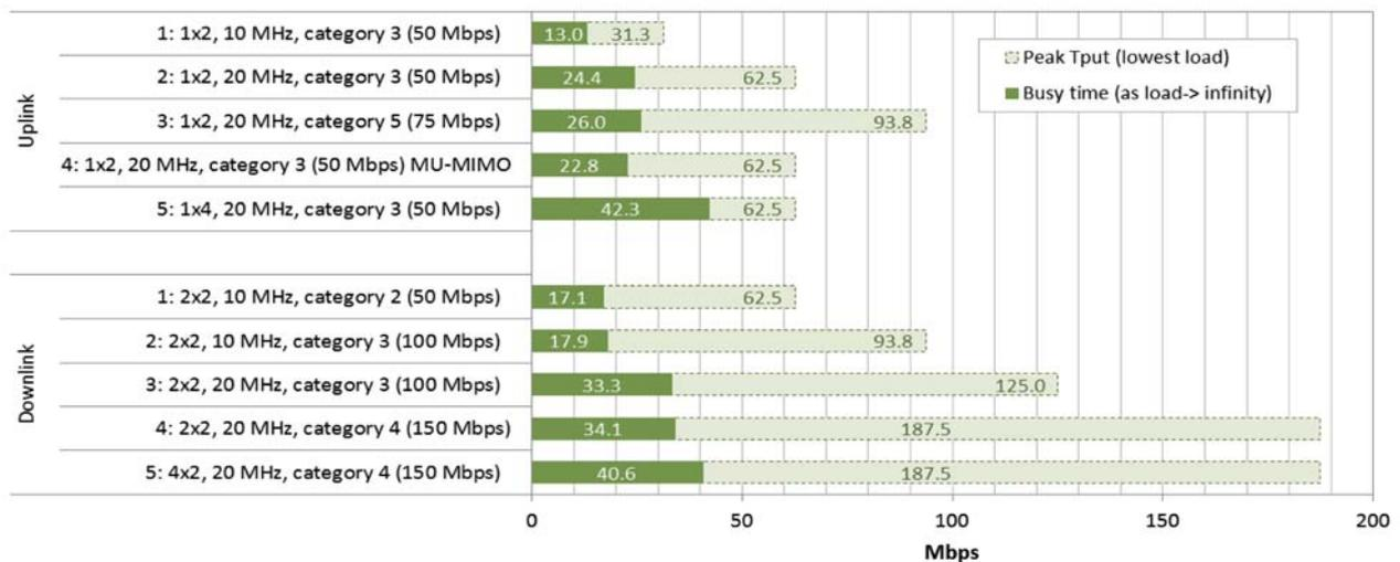
**Figure 13: Backhaul Traffic Characteristics for LTE Small Cells in various configurations**
