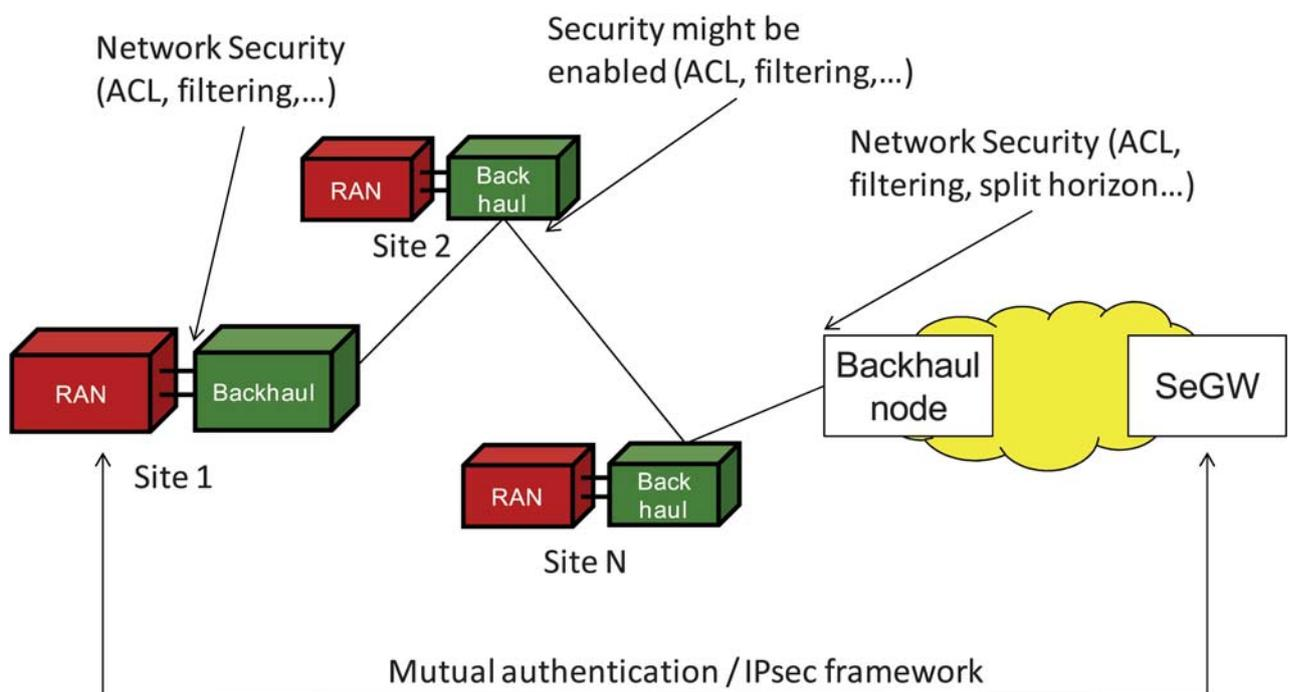
**Figure 17: Security implementation for the “Two box” approach**
