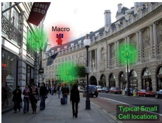
**Figure 8 Typical Small Cell locations**
