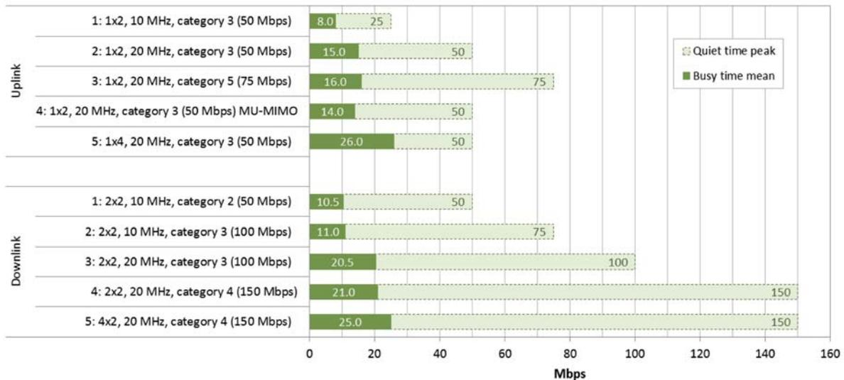
**Figure 10 Mean and Peak User Plane Traffic per Cell for different LTE Configurations, source NGMN [1]**
