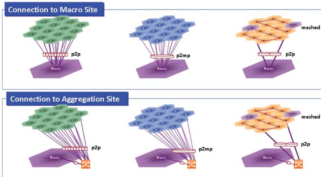
**Figure 3: Basic connectivity options when using an existing macro cell layer**
