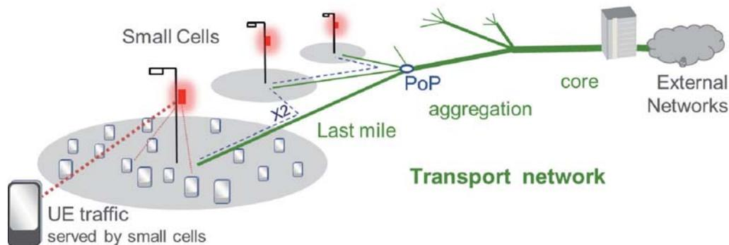
**Figure 1: Abstract View of Small Cell Backhaul with Definitions for Key Nodes and Concepts**
