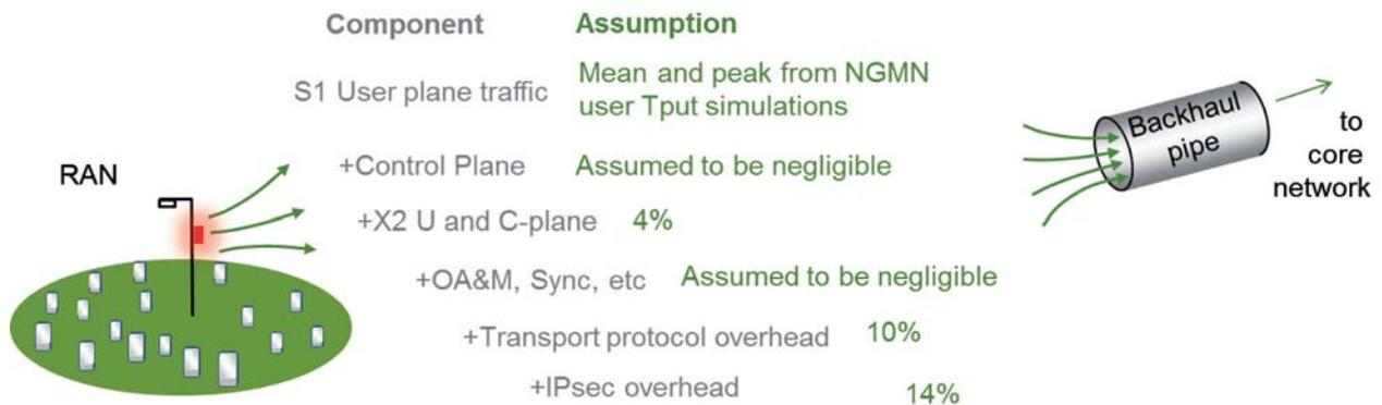
**Figure 9: Components of LTE backhaul traffic and assumptions for overheads**
